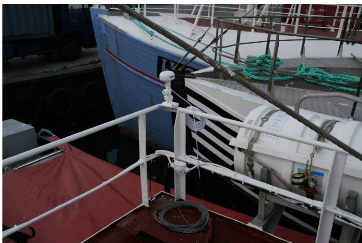
Figure 4. GPS receiver installed in the rigging of a gillnet vessel away from other antennae and radars (left), and a close up photograph of the mounted GPS.
