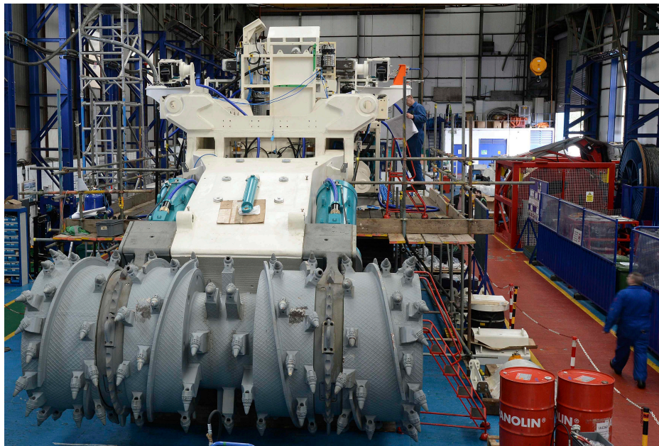
Cutter (AC) - cuts material on uneven surfaces; benching the site
