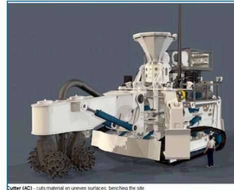
Cutter (AC) - cuts material on uneven surfaces; benching the site
