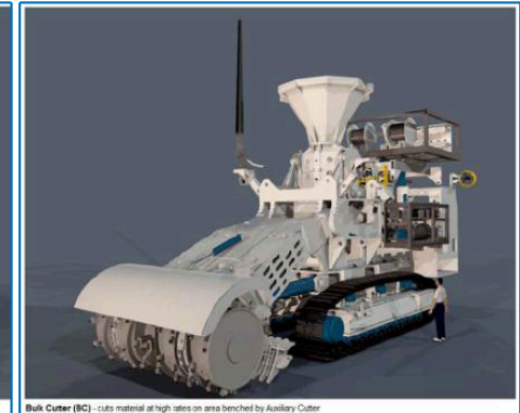
Bulk Cutter (BC) - cuts material at high rates on area benching by Auxiliary Cutter
