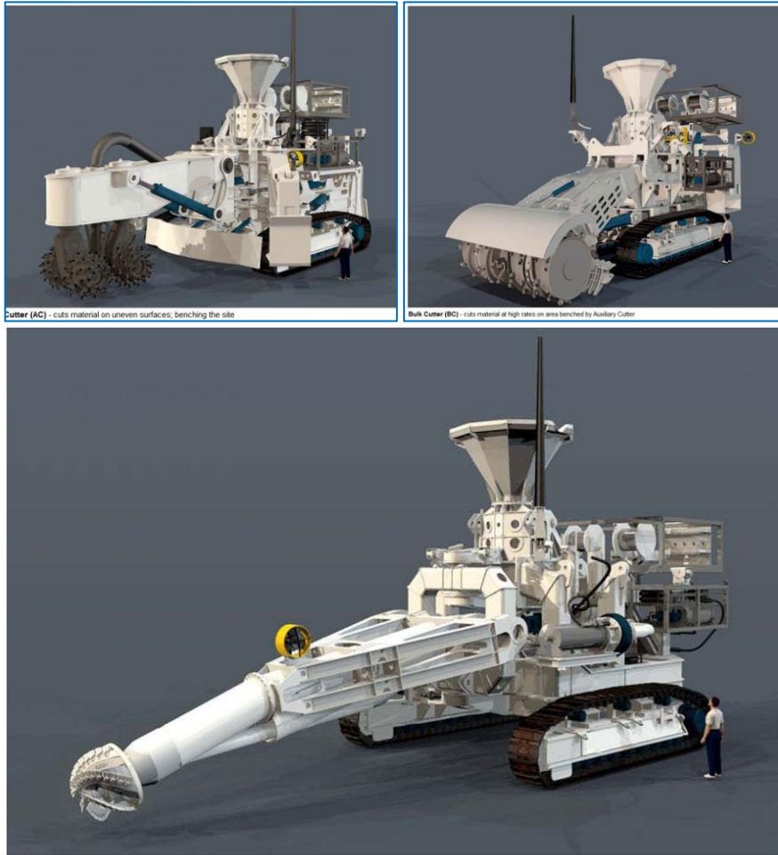
Collecting Machine (CM) - collects cut material with seawater, pumping and transfers the slurry to the RALS
