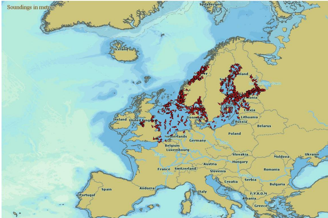
Figure 6-5: Plot of the vessels detected from satellite AIS with on-board processing, Amsterdam to Trondheim capture area.
