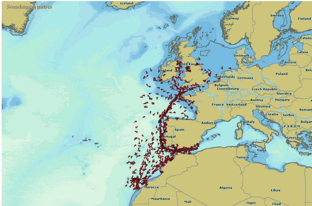
Figure 6-19: Plot of the vessels detected from satellite AIS with on-board processing, Amsterdam to Malaga capture area.
