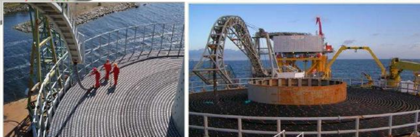
Cable loading & unloading at sea
