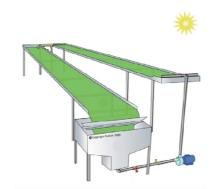
Schematic diagram of a cascade where a thin layer (ca. 1 cm) of suspension flows along declined surface
