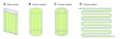
Examples of common closed photobioreactor geometries.
