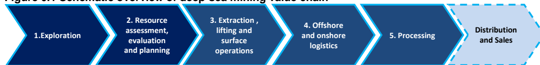
Figure 0.1 Schematic overview of deep-sea mining value chain
