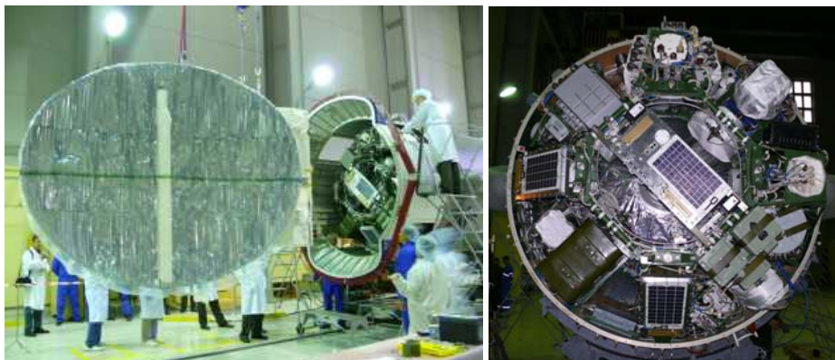
Figure 19: Overview of Rubin-7 spacecraft accommodation on Cosmos-3M launch vehicle
