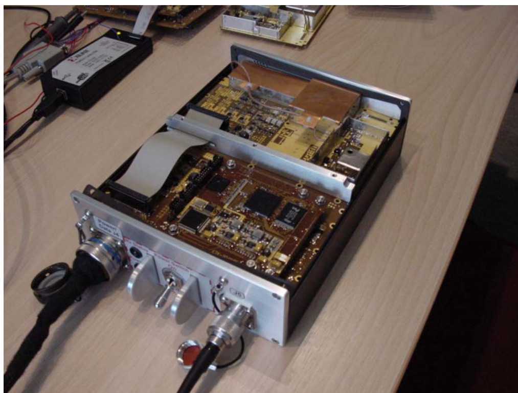
Figure 8: LuxSpace second generation AIS receiver
