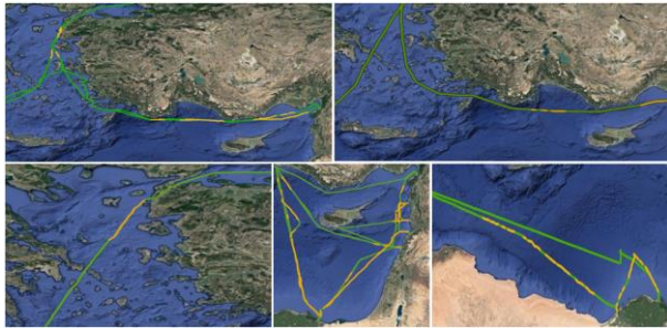
Figure 58. Examples from the gap-filling process. The original trajectory is depicted in green, while the reconstructed segments during the gaps are in orange.
