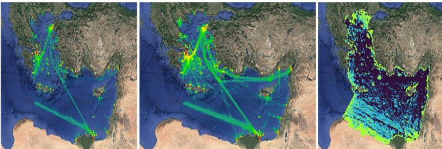
Figure 61. Density maps for the month of October for all vessel types, from Sat AIS data (top), for an improved dataset using the gap filling process (middle) and the difference map
