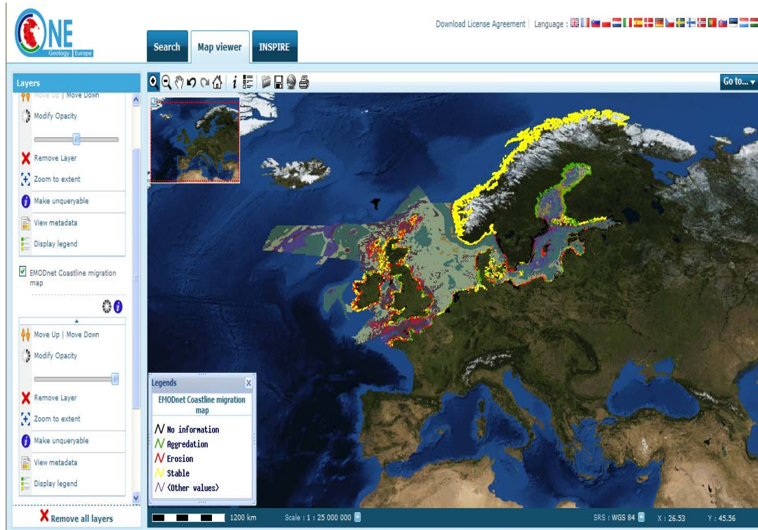
Figure 12. Coastal behaviour, based on the EUROSION database on coastal erosion and sedimentation (includes data outside the EMODnet-Geology study area) in the OneGeology-Europe portal.
