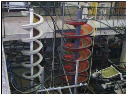
Figure 7.12 Two spiral concentrators
