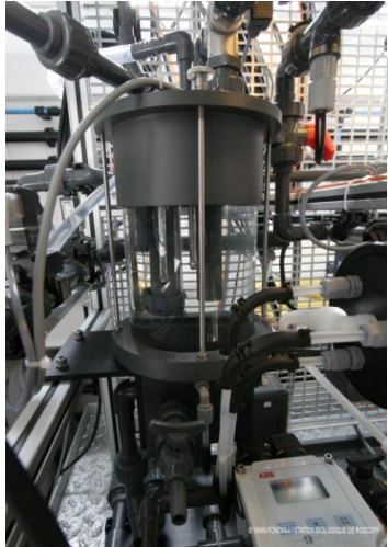
A Ferry Box system, installed onboard MV Armorique (Brittany Ferries). (© Yann Fontana / Station Biologique de Roscoff)
