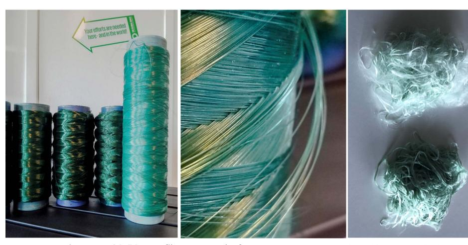
Approx. 30-50 tex fibers - made from: 100% OceanIX rPPC and OceanIX rHDPE (30 tex = 300 gram per 10km fiber)
