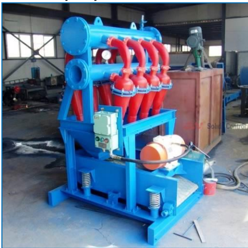
Figure A.4.7.16 A series of hydrocyclones
