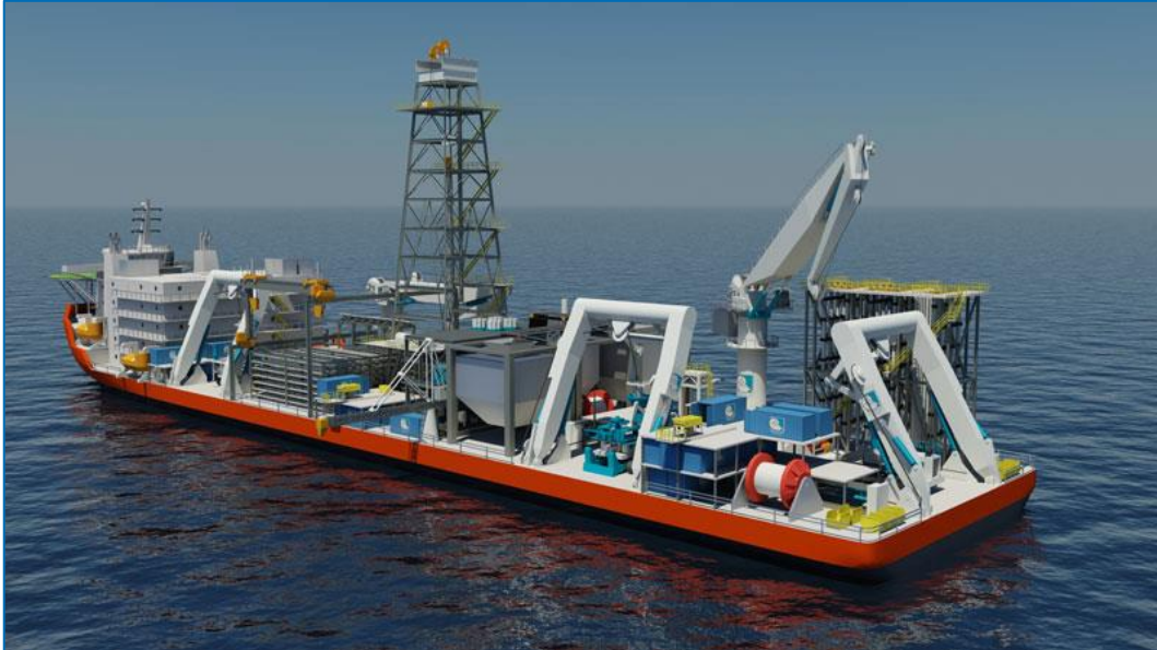
Figure A.4.5.15 Production Support Vessel
