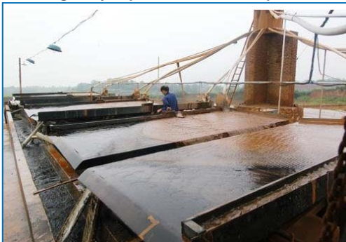
Figure A.4.7.15 A set of gravity separation tables in operation
