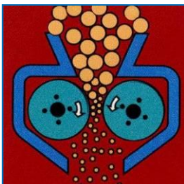
Figure A.4.7.5 Roll crusher
