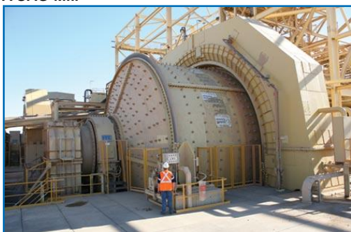
Figure A.4.7.9 A SAG-Mill
