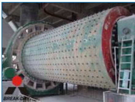
Figure A.4.7.8 Ball Mill
