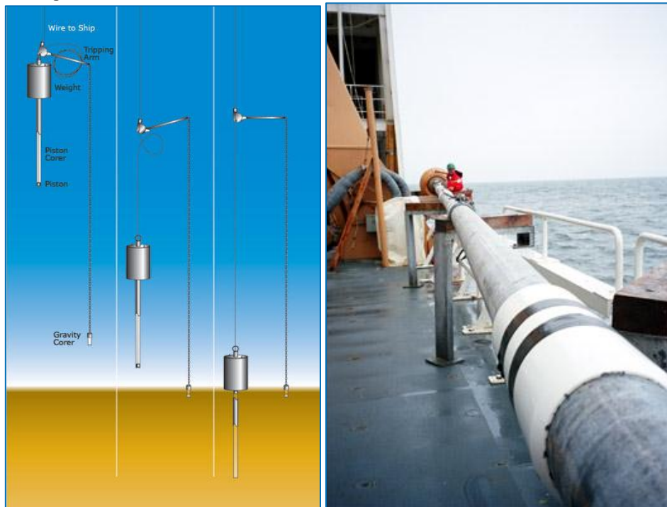
Figure A.4.4.5 Piston coring mechanism
