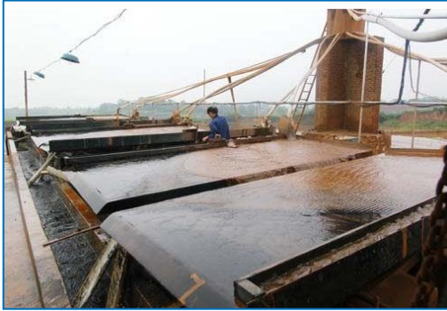
Figure A.4.8.15 A set of gravity separation tables in operation
