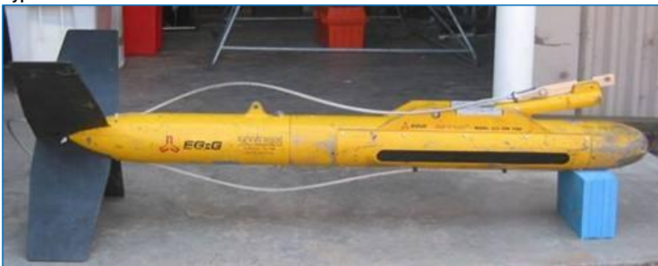
Figure A.4.3.4 Typical side-scan sonar fish
