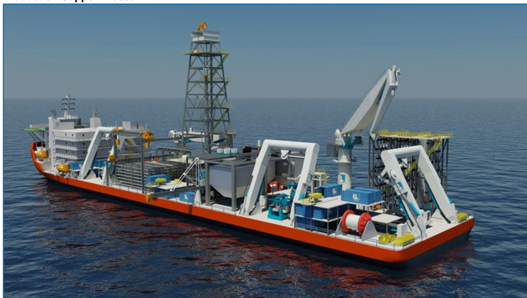
Figure A.4.6.15 Production Support Vessel
