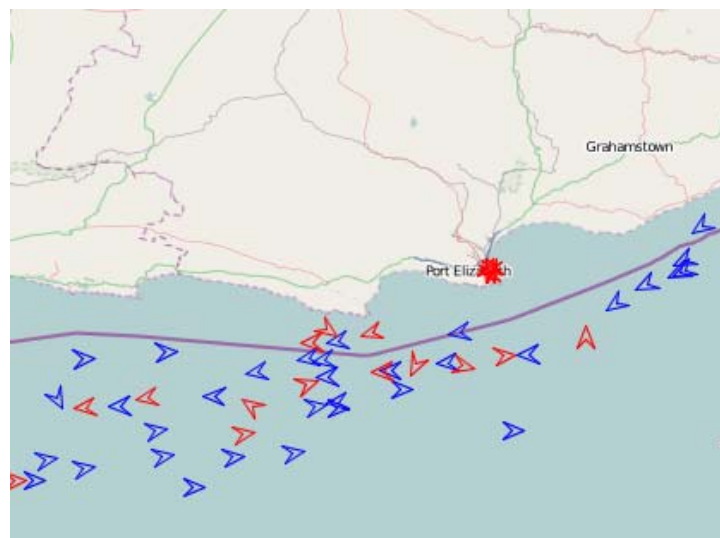
Figure 3: Overlay of LRIT and S-AIS position reports along the South African Coast
